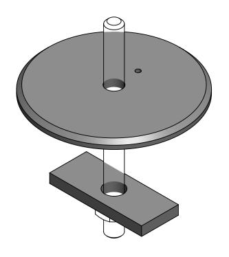
10 MM DIA HOLE TO BE DRILLED ON THE DESK SURFACE TO INSTALL GROMMET CLAMP.
